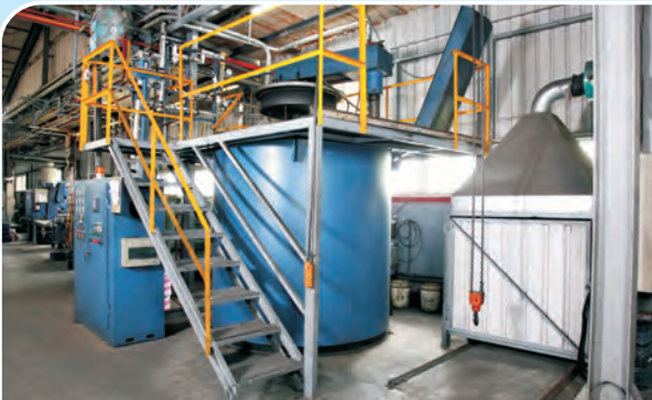
黑化爐 Pressurized Steam Treatment Furnace
