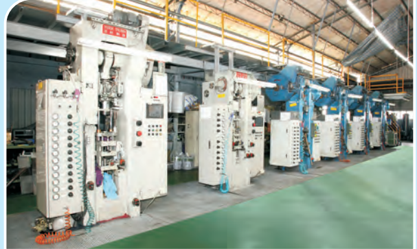
成型機台 6 ~ 160 Tons Mechanical Compacting Machines
