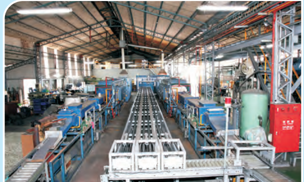
自動化燒結爐 Automated Rapid Cooling Furnace
